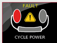
Left Pad Fault
